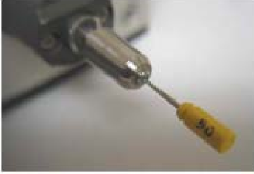
Figure 3 -Root canal reamer inserted into the pipette spigot.
