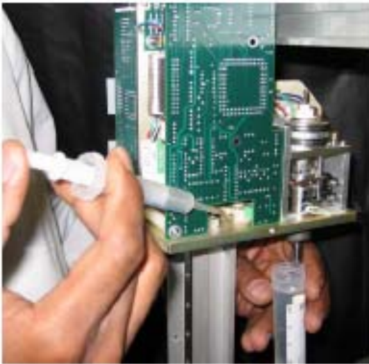
Figure 4 - Injecting alcohol into the tubing from the sensor end.
